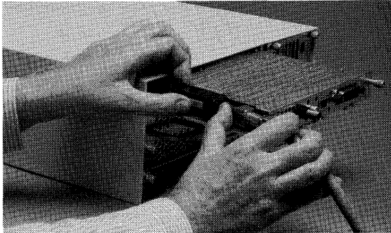
Connecting Cable to Interface Card
